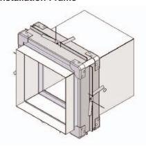
The HEVAC Installation frame allows the damper to be built directly into masonry walls and concrete floors. It allows the damper to expand in fire conditions, thus maintaining the integrity of the wall or floor.
