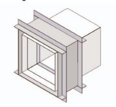
The Sleeve and Angle frame installation can be used as an alternative to the HEVAC frame. A sleeve can be factory fitted to the damper and additional angles are fixed to the flange which sandwiches the wall at the same time.
