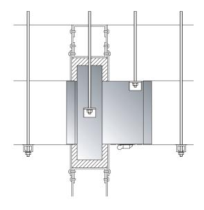
**Note:** It is important that the appropriate installation accessory is used to suit on site requirements. For a fire barrier to maintain its integrity in a fire situation the damper must be securely installed and the damper should be independently supported. Advanced Air are able to discuss your requirements and help with selections.
