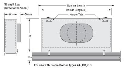
Plenum Height (HS): One Slot 250mm, Two Slot 400mm
